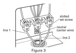
Use this method only if local codes permit connecting ground conductor to neutral supply wire.
